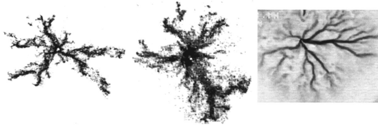
FIG. 7. Branching topology obtained in unstable pumping of water from sand particles (with a size of \sim 250 \mu\text{m} and flow rate of 8 ml/mn on the left) and from spherical glass beads (with a size of \sim 200 \mu\text{m} and flow rate of 4 ml/mn in the middle and size of \sim 40 \mu\text{m} and flow rate of 0.08 ml/mn on the right).
